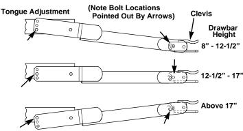
It is important that the TD be operated in a level position. Leveling can be accomplished by adjusting the implement hitch to the tractor draw bar height and leveling the mowerframe by use of the adjustable jackstand.
